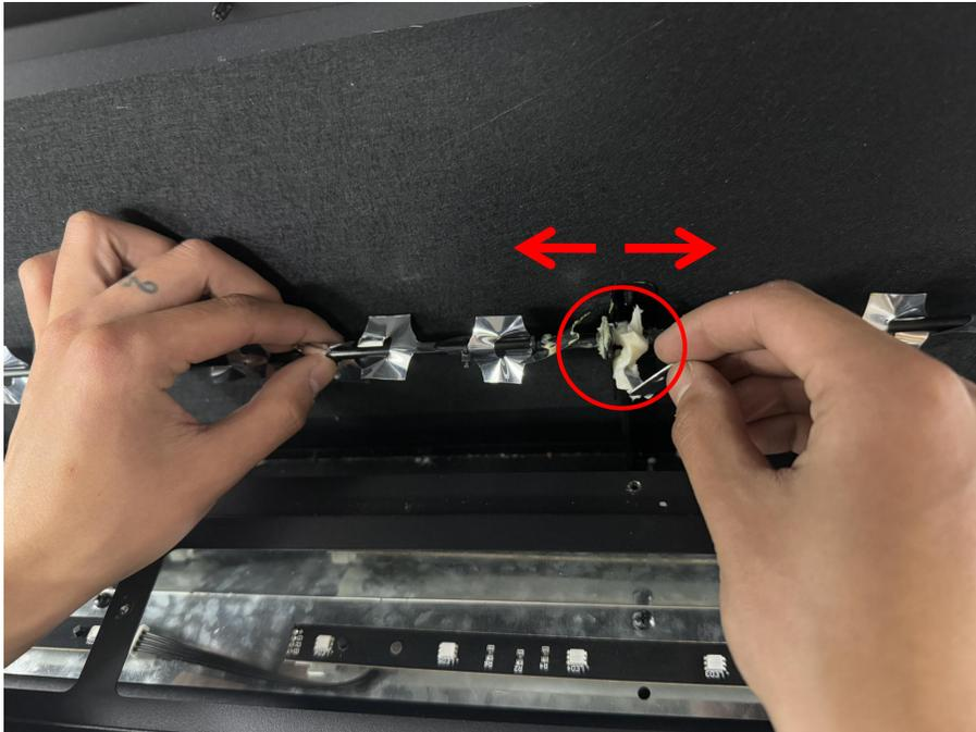
Grease inside the rubber center grommet
