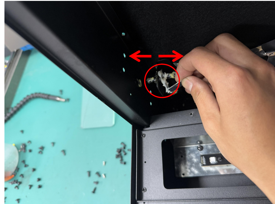
Grease inside the rubber grommet on the left
